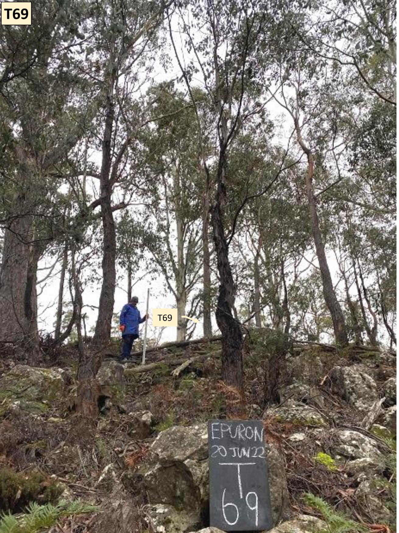
**Plate T69-1.** View west and steeply upslope, near the top of the east-facing hillside with a heavy float of dolerite cobbles and boulders, and isolated outcrops of high strength rock. T69 is located about 50m west.
