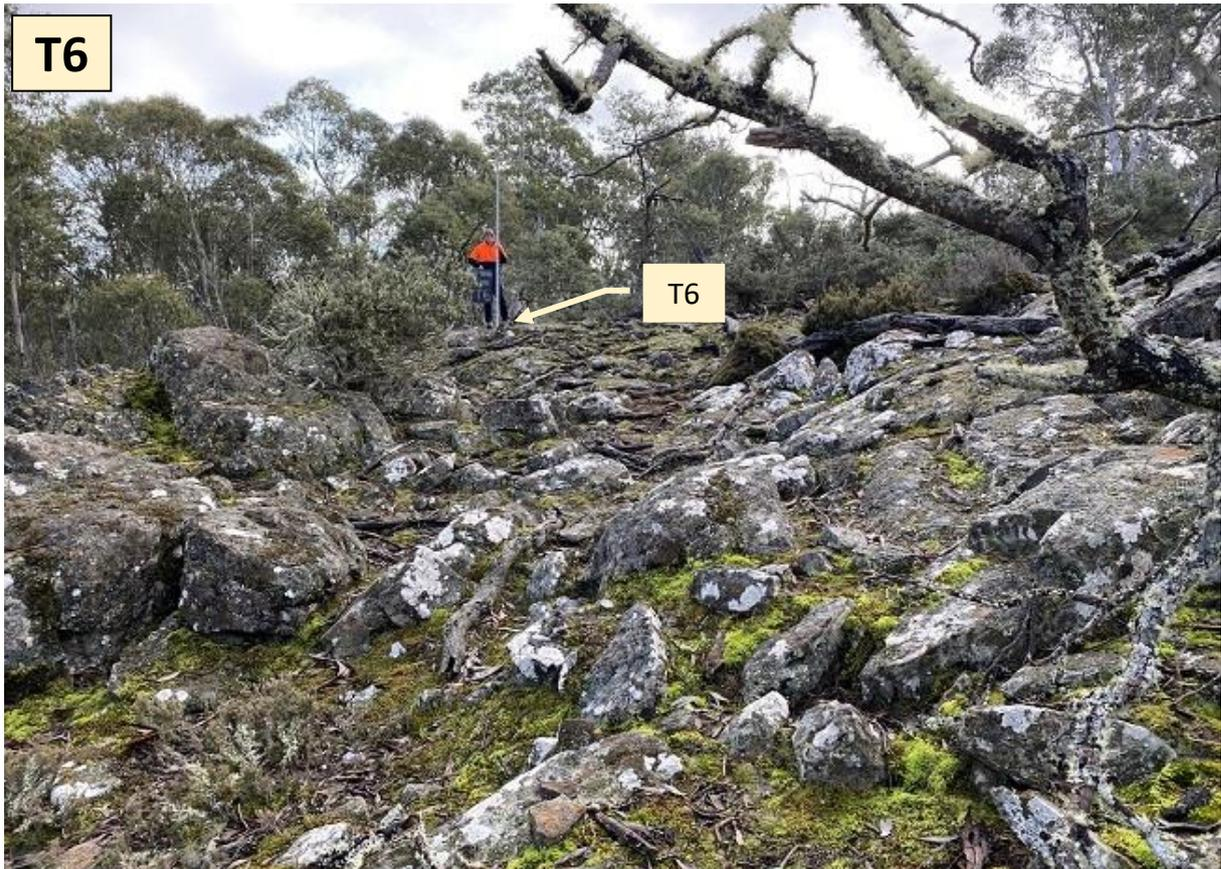
**Plate T6-3 (above).** View north and slightly upslope towards T6. Dolerite cobbles and boulders float litter the ground, and outcrops of exfoliated high-strength bedrock are common. The staff is 3m high.
