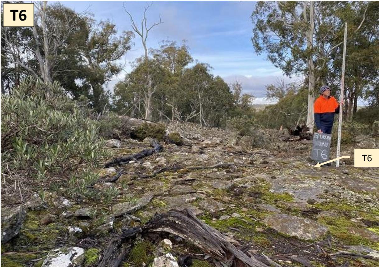
Plate T6-1 (above) and Plate T6-2 (below). View south to T6. Dolerite cobbles and boulders float litter the ground, and outcrops of exfoliated high-strength bedrock are common. The staff is 3m high.
