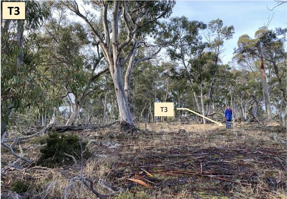
**Plate T3-1 (above).** View north near proposed tower T3, on the almost flat crest of a broad spur trending NNW – SSE; the ground slopes gently in these directions at angles in the 0–5° range. Slopes steepen to up to 30° and more along the sides of the ridge. The staff is 3m high.
