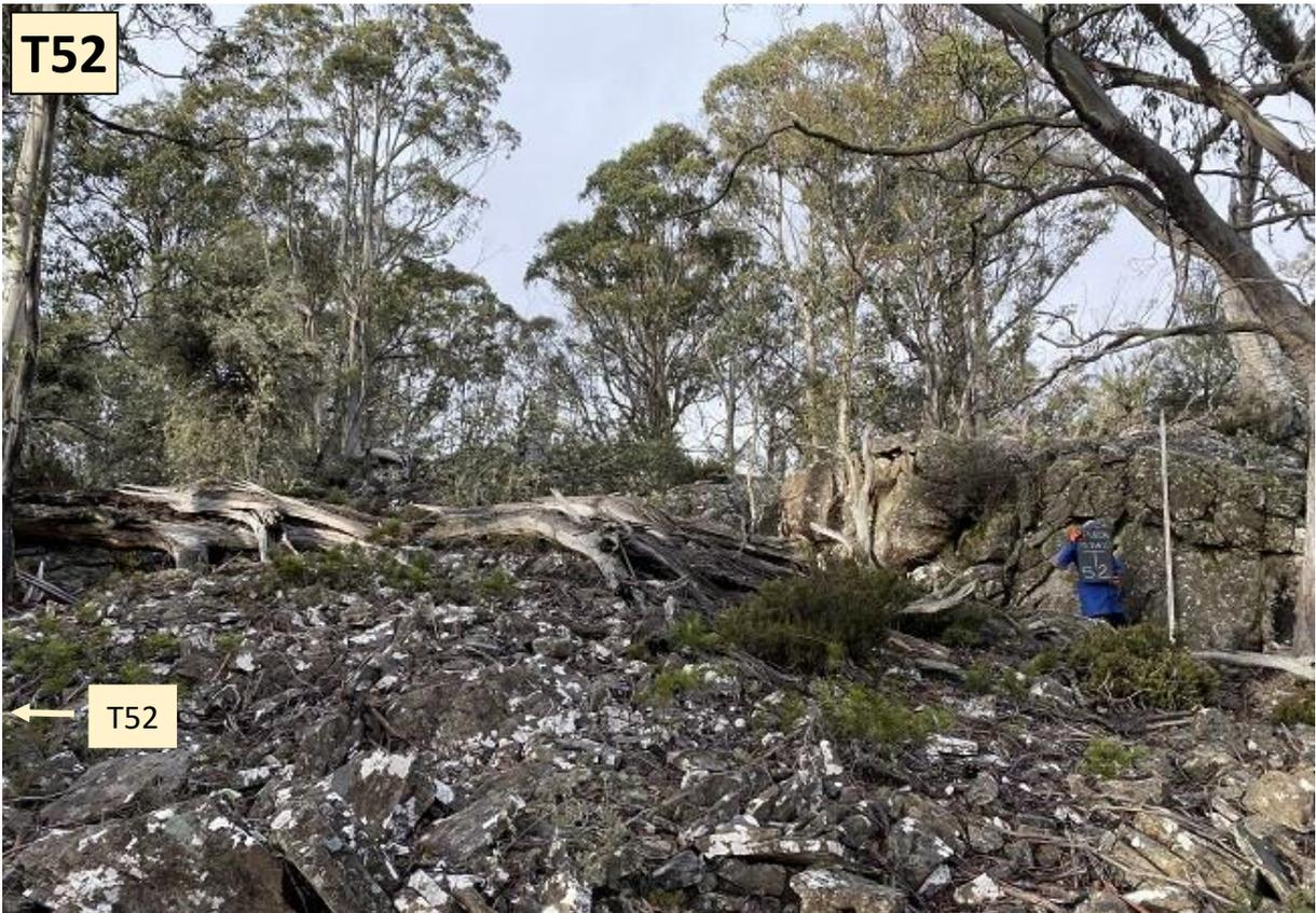
**Plate T52-3 (above) and T52-4 (below).** View southeast. Site T52 is to the left. A float of approx. 80% cover of dolerite cobbles and boulders on gently rising ground. The outcrop of high strength dolerite with subvertical north-south jointing at right (above) and centre (below) falls away steeply at the rear in 10- – 15m high cliff sections. The staff is 3m high.
