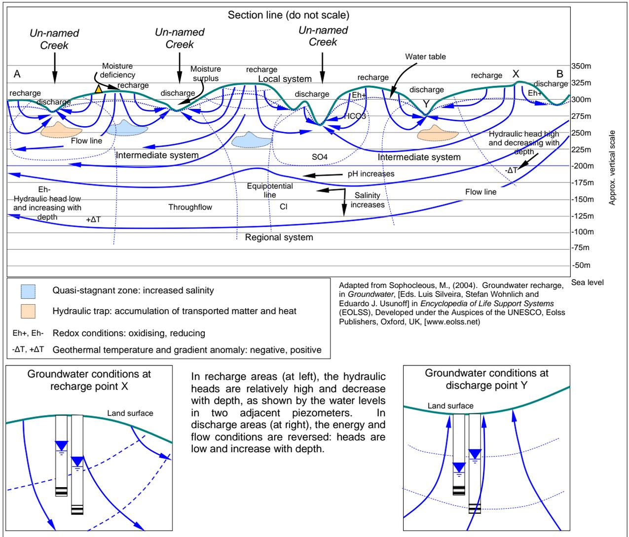
Figure 5. Fundamentals of groundwater hydrology in a gravity-driven groundwater system like that in the study area. Vertical exaggeration for the top section is about 5.
