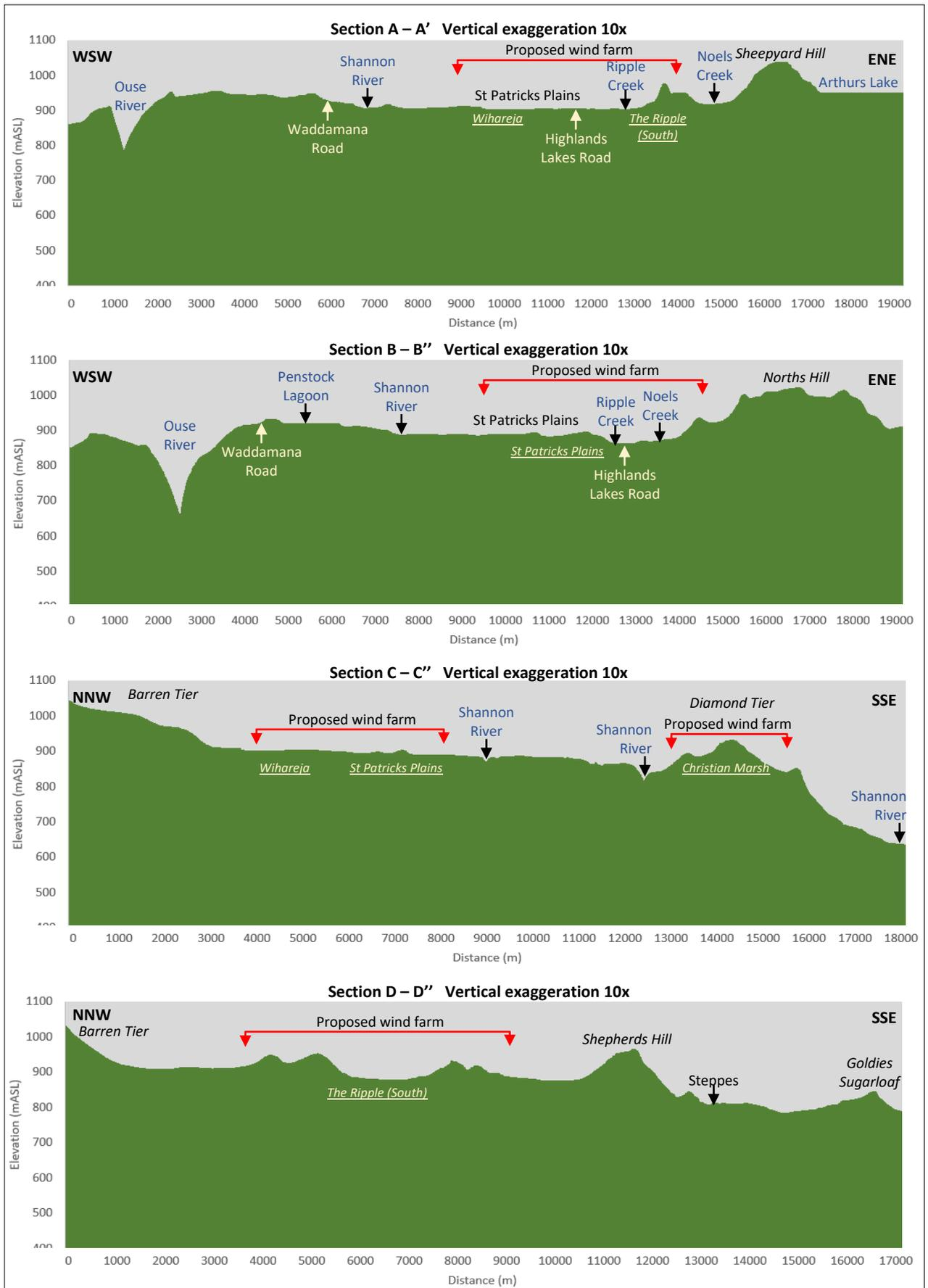
Figure 3. Topographic profiles (vertically exaggerated 10 times) along section lines A - A' to D - D' depicted in Figure 2.
