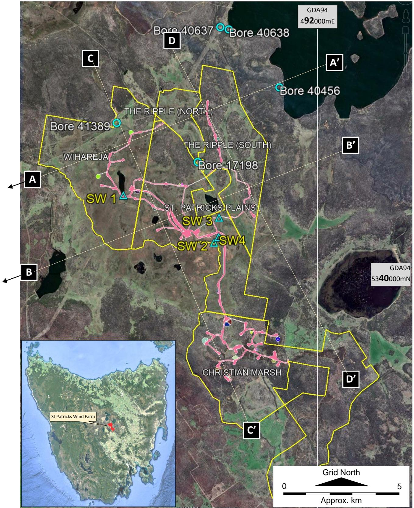
Figure 2. St Patricks wind farm infrastructure (pink lines) on St Patricks Plains. Yellow lines are property boundaries. Also shown are hydrogeological cross section lines A - A'.....D - D'. Recorded groundwater bores (Bores 41389 and 17198) were pump tested and sampled for this report, and surface water locations SW1, SW2, SW3, SW4 were sampled for this report) Source of base image: Google Earth; image date 28 October 2019.
