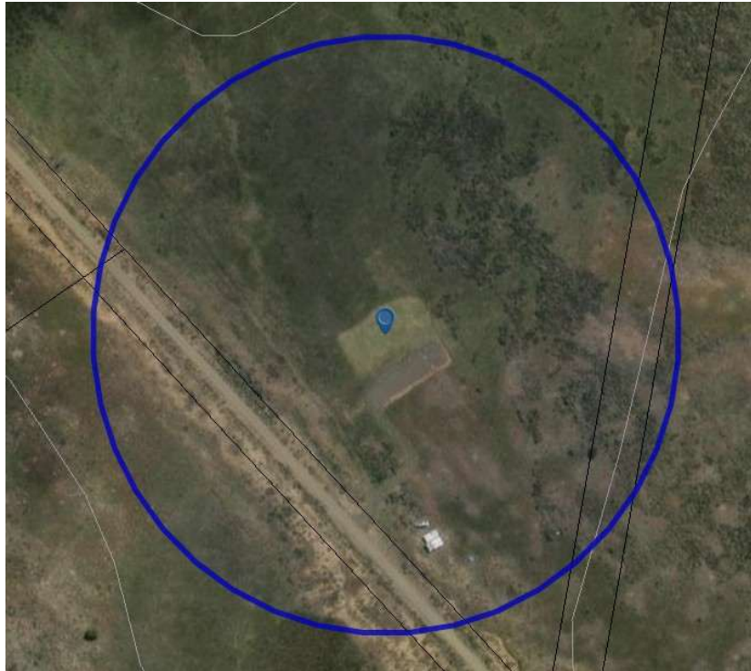
Aerial view showing 120m radius from site of proposed dwelling. Landscape dominated by highland sedgeland and heathland, assessed as vegetation classification 'Group C Shrubland' as per table 2.3 of AS3959.
