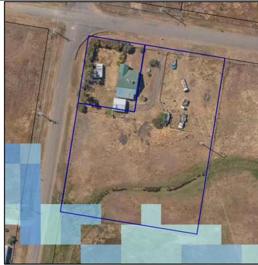
Figure 4 – 1% AEP (+CC) Overland Flood Mapping - Subject site (highlighted in blue). Source: LISTMAP
