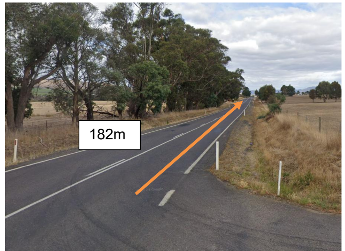
Figure 07: SISD To 182m from the Intersection
