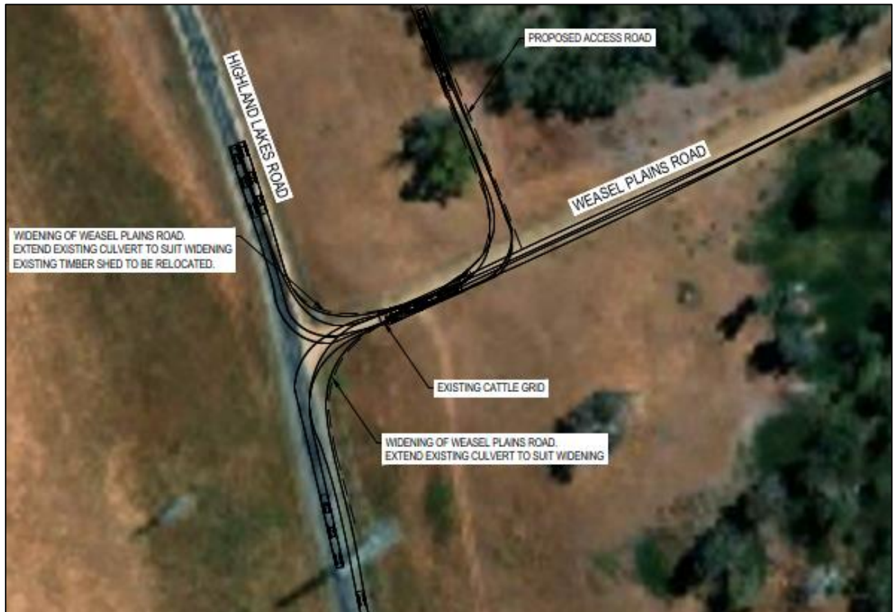
Figure 25: swept paths for B-double trucks entering and exiting Weasel Plains Road and the proposed site access road
