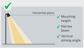
**Figure 3:** Application of mounting height and vertical aiming angle to control light spill
