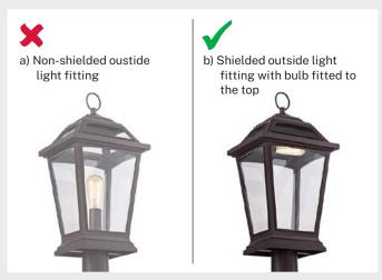
**Figure 9:** Exposed bulb that allows light to shine in all directions and a fitting designed to minimise light spill by only allowing downward projection of light
