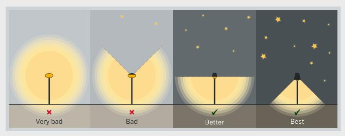
Figure 7: Examples of upward light spill ranging from the worst case (left) to the best case (right)
