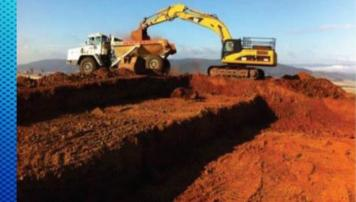
Picture courtesy of Australian Bauxite Limited. Surficial bauxite mining at Campbell Town, Tasmania, 2015.
