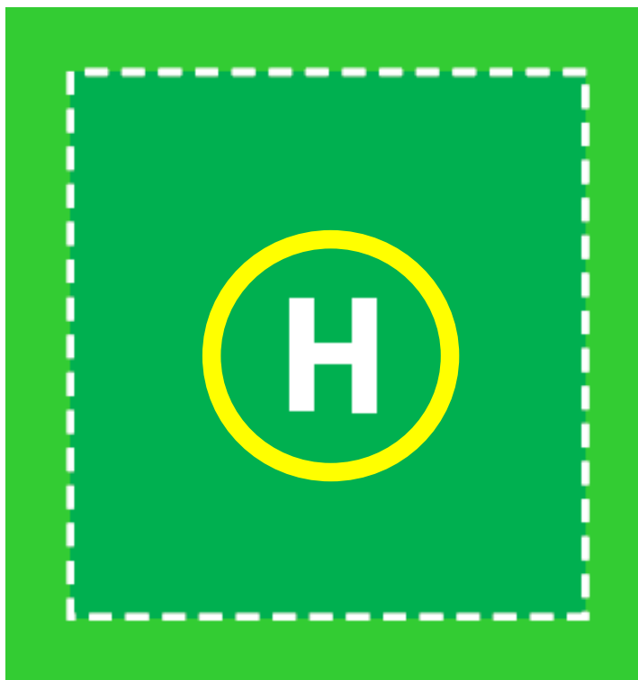
Figure 1 – Secondary HLS: A 1.5 \times D FATO with additional 0.25 \times D Safety Area (Total area is 2 \times D ). Also showing 'H', FATO perimeter and 0.5 \times D Touchdown/Positioning Markings (TD/PM).
